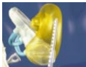
Electrode array with Stylet is introduced into the Cochlea
